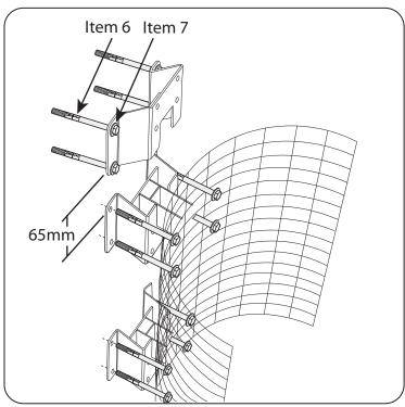
Fix the cage to the wall using the Anchor Bolt (Item 6) and Washer (Item 7) ensuring the cage is located in the correct orientation, at the correct height and level. Next, secure the Orbis Wall Mounting Bracket (Item 5) 65mm above the upper Cage Wall Mounting Bracket. NOTE// The Orbis Wall Mounting Bracket is fixed upside down compared to the Cage Brackets.
