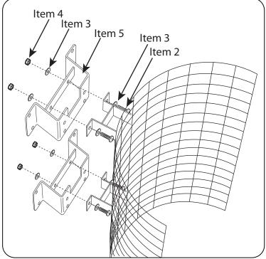
Take the rear cage and align the fixing holes with the two holes on the inside of two Wall Mounting Brackets (Item 5) in the orientation shown. Secure in position using the Screw (Item 2), Washer (Item 3) and Nut (Item 4) provided.
